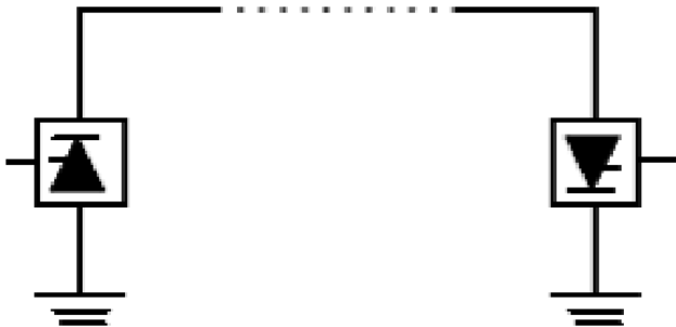
Figure 1 monopole HVDC system
