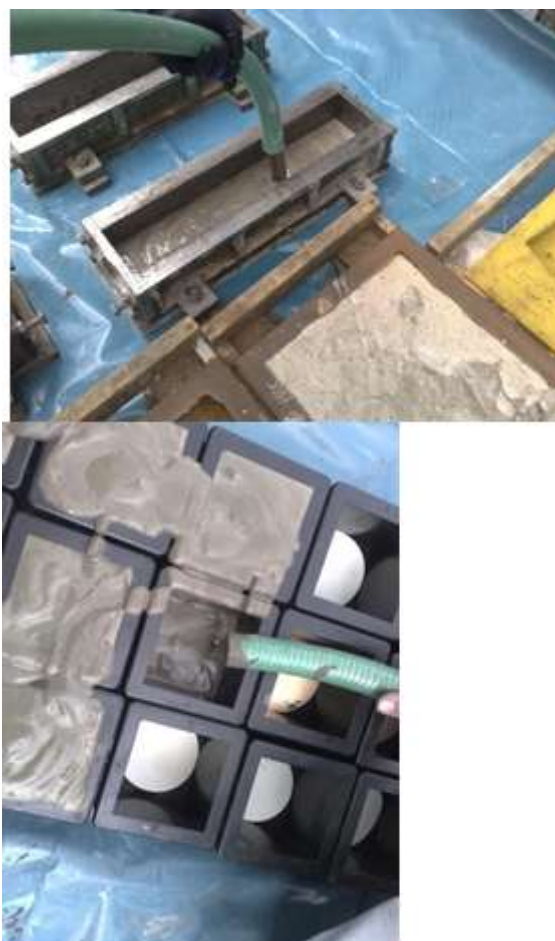
Fig.1 Aer-Tech material being poured in the moulds
